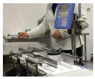
Production line checkweighing at Atlas Putty
